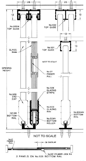
GLASS SIZE FOR DOUBLE PASSING PANELS Height = Opening height less 31mm. Width = Half opening width plus 16mm.
